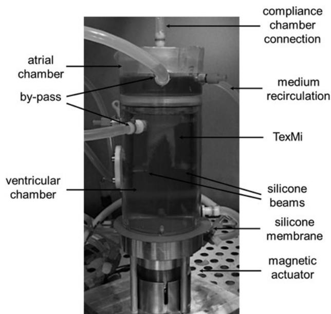
**FIG. 2.** Bioreactor system for conditioning of TexMi. The valve is mounted with the chordae tendineae sutured to silicone beams to enable closing and opening cycles.
